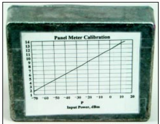
The calibration curve taped to the back of the instrument provides output readings in dBm relative to the meter's 0 to 15 V scale.
