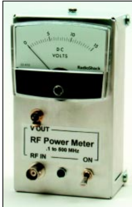
This version of the power meter is built in an inexpensive RadioShack utility box.
